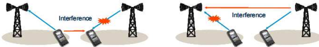
Figure 6. Overview of interference scenarios for FDD and TDD systems
